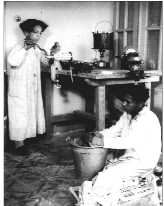
Figure 2. The model makers in Cairo used ‘mangarieh’, a mixture of minced newspaper, local plaster and glue. [Reproduced with kind permission of the Public Record Office.]
